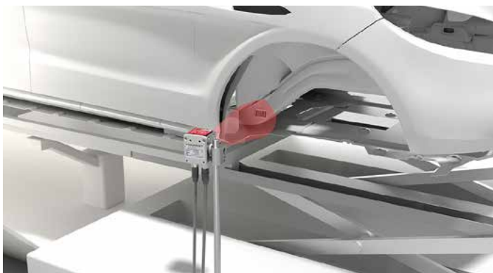
Camera-based code readers using identCHAIN not only provide individual object identification, but also device and status information for each production step.
