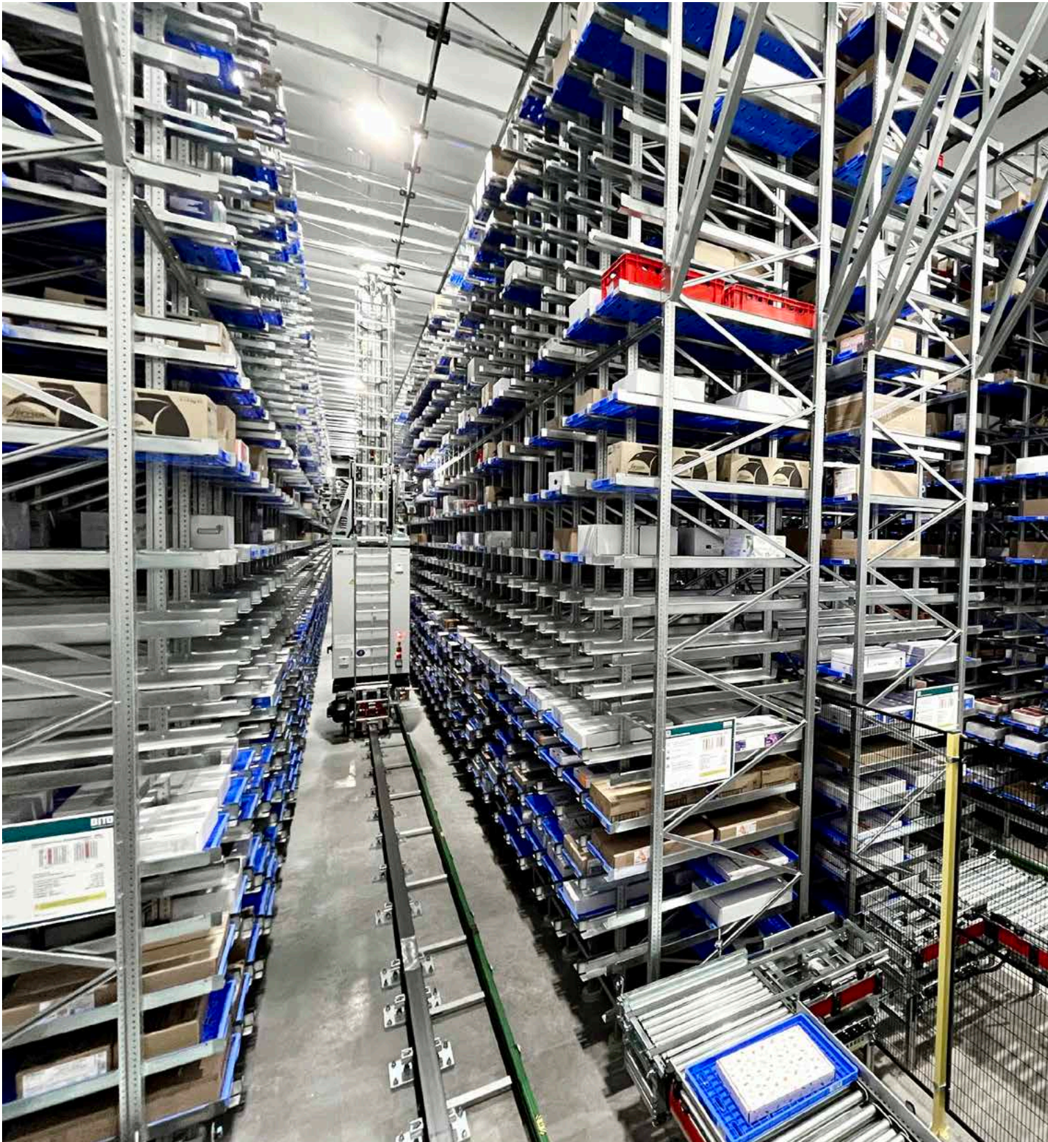
Automated deep-freeze warehouse with over 26,280 tray storage locations
